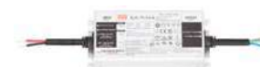
DRIVER - 9621508 Meanwell LED Driver 75 Watt Input: 100-240V AC 3.1A Output: 24V DC IP67 5 Years Guaranty L: 14 W: 6.3 H: 3.2 cm
